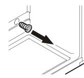
Pull out strain relief device.
