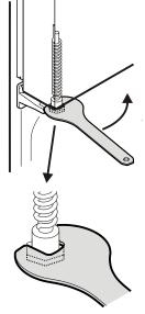
10. Reinstall the middle hinge bracket on the left-hand side.
